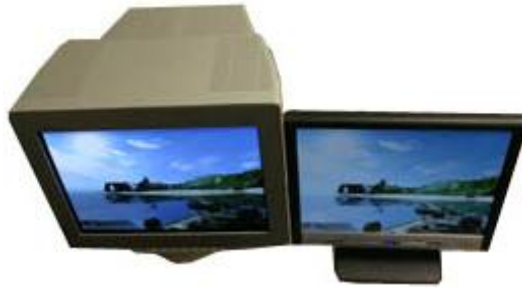
Figure1: a flat panel LCD display is compared with a bulkier CRT
